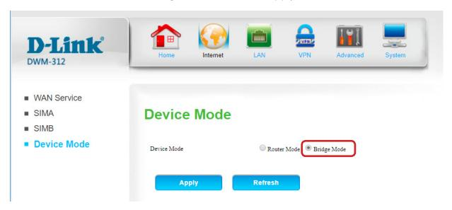
The Setup is complete for DWM-312 in Bridge Mode. See next page to setup Sophos Firewall for failover.
